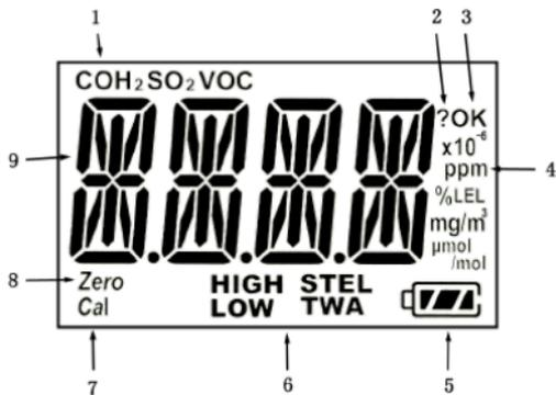
1. Gas name, including CO, H<sub>2</sub>S, SO<sub>2</sub>, or O<sub>2</sub>
