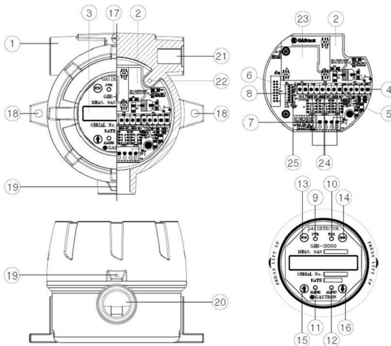
Figure 2. Components of NDIR Point 3000
