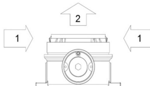
Figure 4. Separation method for Display Part
