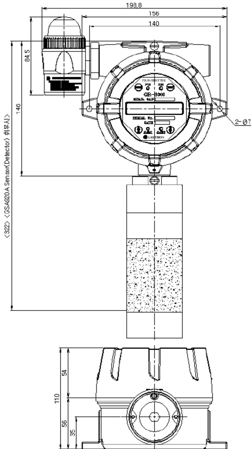
Figure 18. Outline drawing for coupling of NDIR Point 3000 warning light
