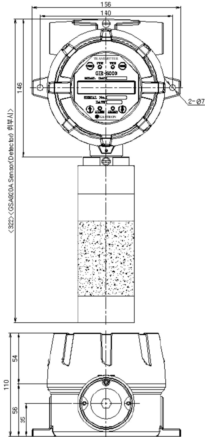
Figure 17. outline drawing for NDIR Point 3000 Standard Type
