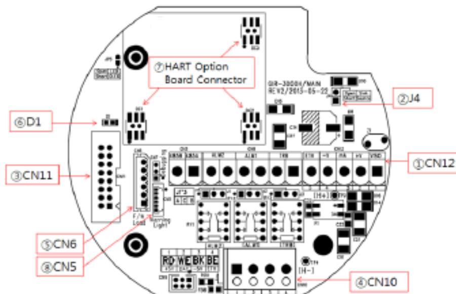
Figure 5. Layout diagram for Main PCB terminals
