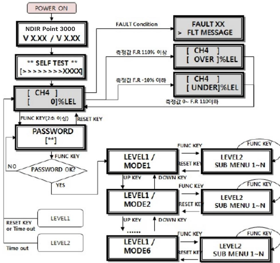
Figure 16. Configuration of NDIR Point 3000 mode
