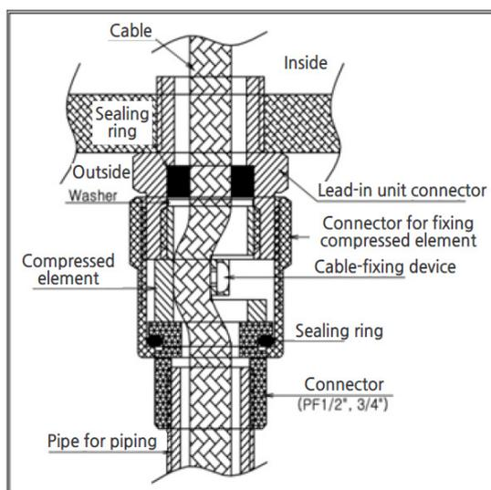
Figure 21. Pressure-resistant packing type
