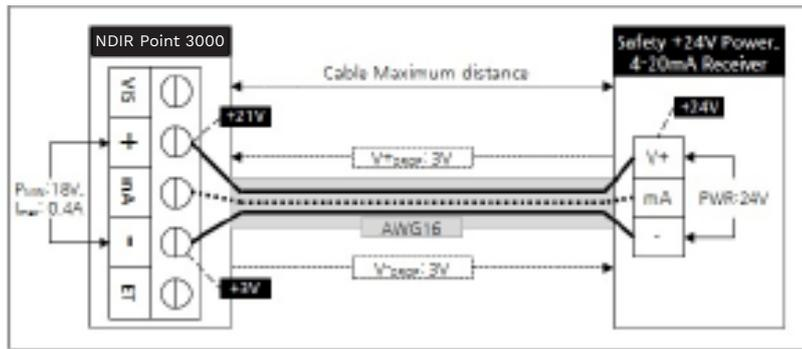
Figure 15. Calculation of length for NDIR Point 3000 installation cable
