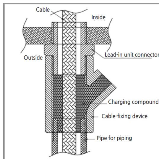
Figure 22. Y Sealing Compound
