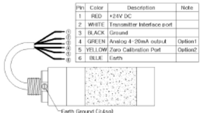
Figure 13. Configuration of connection for GSA920A
