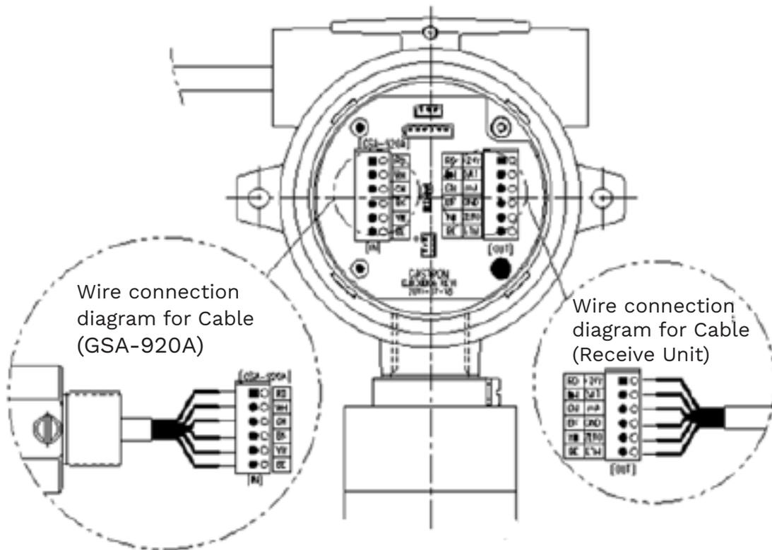
Figure 14. Configuration for GSA-920A Remote Type
