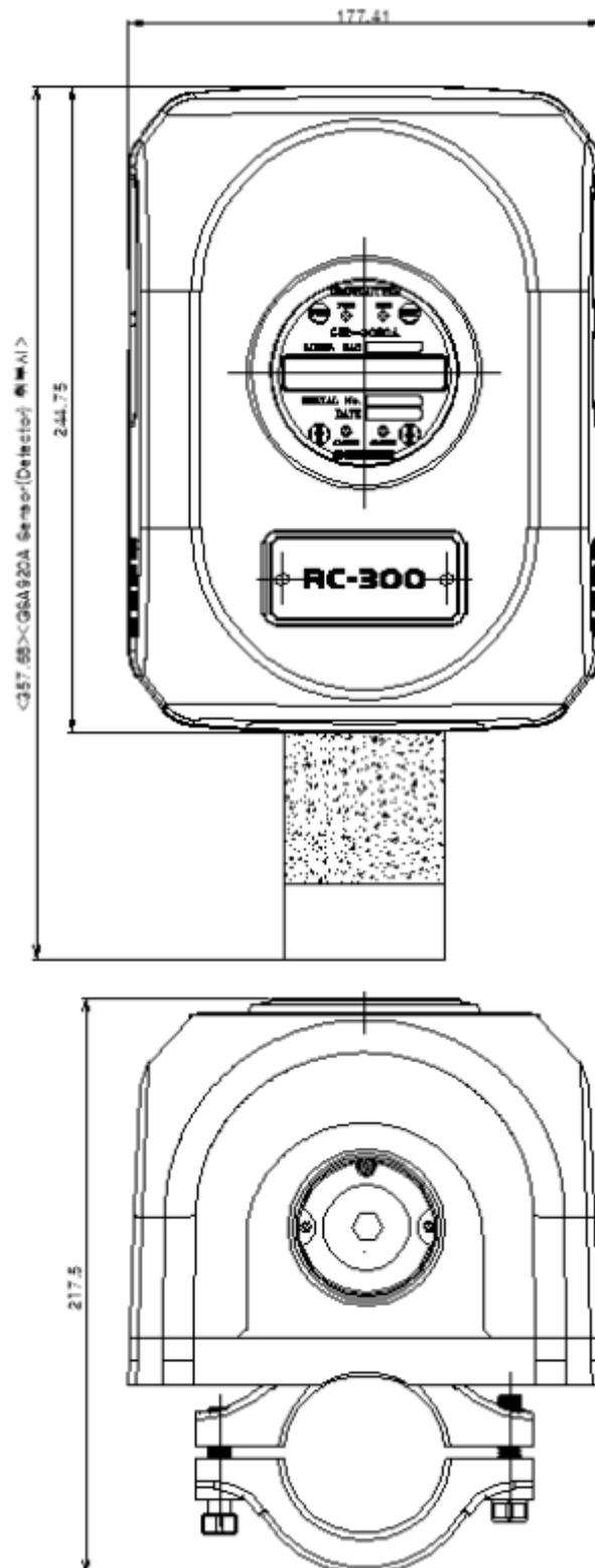
Figure 19. Outline drawing for coupling of NDIR Point 3000 Raincover
