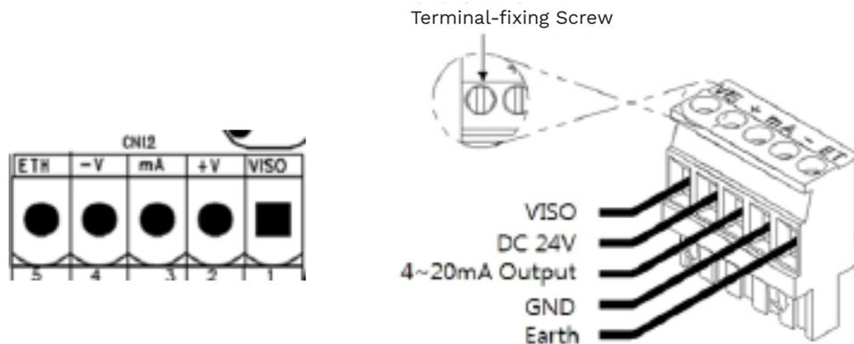
Figure 6. Configuration of CN12 terminal
