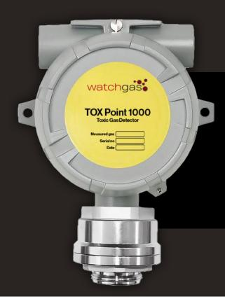
The TOX Point 1000 is a reliable, user-friendly detector for oxygen and toxic gases, built with an explosion-proof design to prevent secondary explosions. It supports 4-20mA output (source or sink) and offers high quality at a competitive price. A built-in FND display allows easy inspection and calibration, which can be performed by a single operator.
