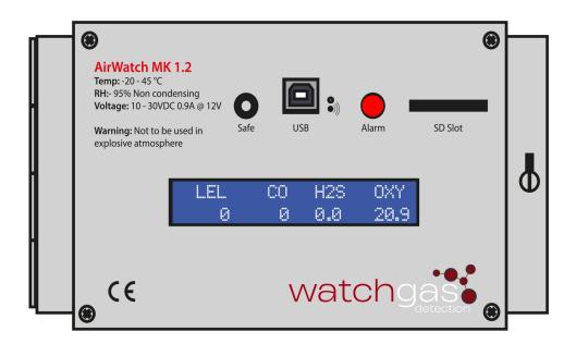
Red LED. The AirWatch alarm is activated. A gas concentration is being detected that is higher than the alarm values, or the pump is blocked (if the pump is blocked "pump Blocked" will be shown on the LCD).
