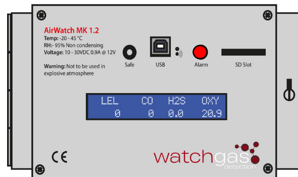
Red LED. The AirWatch alarm is activated. A gas concentration higher than the alarm values has been detected, or the pump is blocked.
