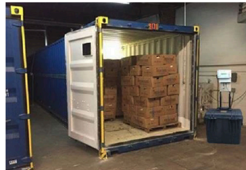
Figure 1: AirWatch GasPod for Shipping Container Measurement
