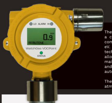
The Stationary Photoionization Detector VOCPoint is a continuously measuring detector for volatile organic compounds (VOCs) with an ionization potential <10.6 eV. (New: optional with 11,8eV lamp) The use of new technologies for the excitation source and the sensor allows a high stability of measurement and longer maintenance intervals. An integrated active carbon filter and the circuit sampling an automatic fresh air setup and automatic calibration are controlled.
