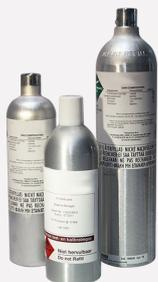
Calibration Gas for CO<sub>2</sub> (Span) and N<sub>2</sub>
