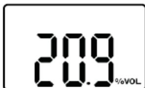
In measuring mode, gas concentration will appear on the screen. Oxygen concentration in percent by volume (%vol) and toxic concentration is displayed in parts
