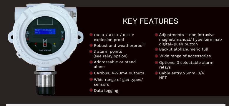
The XDIwin–F1+ Gas Sensor is capable of utilising a wide range of sensor cell types offering an unmatched number of gases that may be monitored. Standard 4~20mA signaling with CANbus address enables the sensors to be networked via the WatchGas Combi control system or customer preferred monitoring systems. Adjustments to menu settings and readings may be made by a single magnet without the removal of the enclosure lid, alternatively push button adjustment is accessible by removing the lid.
