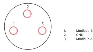
Pin out of the 3 pins modbus connector
