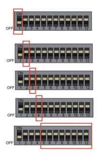
DIP switch 1 ON = digital / Modbus input
