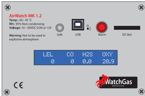
Red LED. The AirWatch alarm is activated. A gas concentration higher than the alarm values has been detected, or the pump is blocked.
