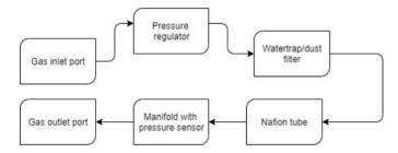
Figure 3: Schematic structure of the gas flow
